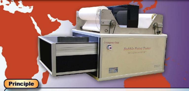
Capillary flow porometry is used to characterize the pore structure. In this technique flow rate of an inert gas through the sample is measured in dry conditions as a function of differential pressure. The sample is wetted using a wetting liquid and the flow rate of the inert gas through the wet sample is measured as a function of differential gas pressure. Differential pressure yields pore diameter.
