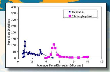
often used as fuel cell components can determine the performance of the fuel cell, and reaction rate of reactants is governed by the surface area of through pores. The Fuel Cell Porometer is designed to measure all the relevant pore structure characteristics of fuel cell components.
