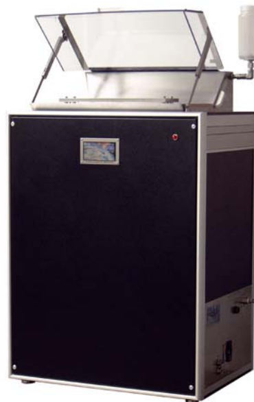
Fig.1 The PMI liquid permeameter used in this study.
