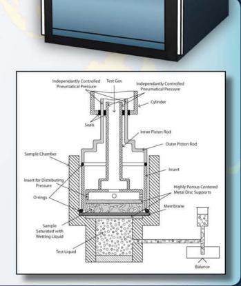
Compression Liquid Extrusion Porosimeter
