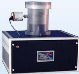
Permeameter High and Low Gas Permeability
