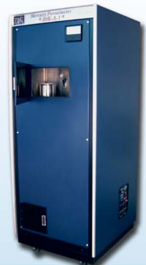
Mercury / Non-Mercury Porosimeter Pore Volume & Distribution
