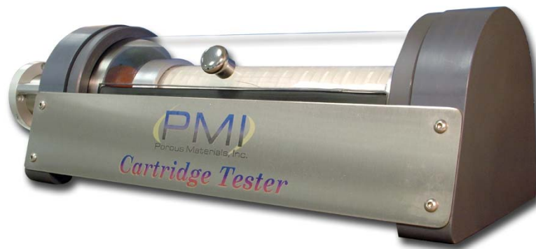
Figure 1. Sample chamber for testing filter cartridges.
